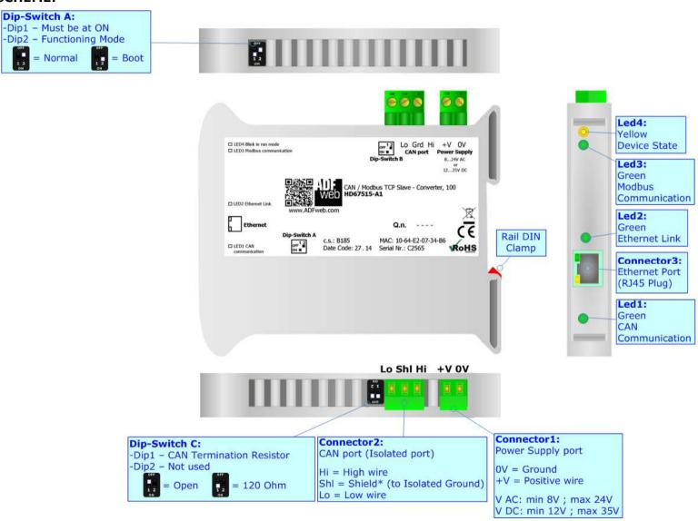
Figure 1a: Connection scheme for HD67515-A1
