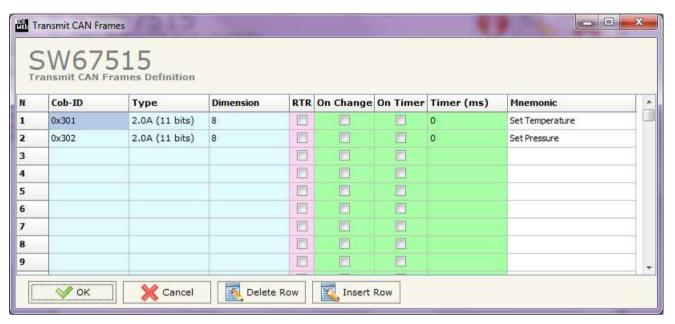
Figure 6b: "Transmit CAN Frame Definition" window
