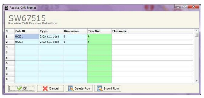
Figure 4b: "Receive CAN Frame Definition" window
