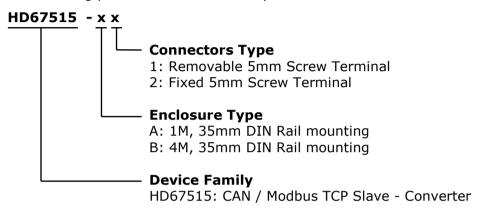
Order Code: **HD67515-A1** - CAN / Modbus TCP Slave - Converter ( Housing type: A, Terminal Blocks Connectors )
