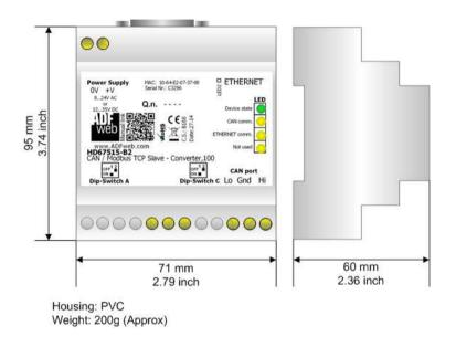
Figure 11: Mechanical dimensions scheme for HD67515-B2
