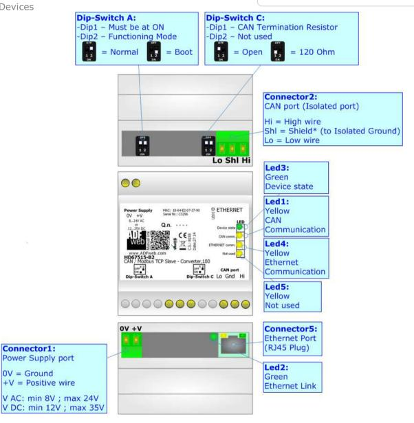
Figure 1b: Connection scheme for HD67515-B2
