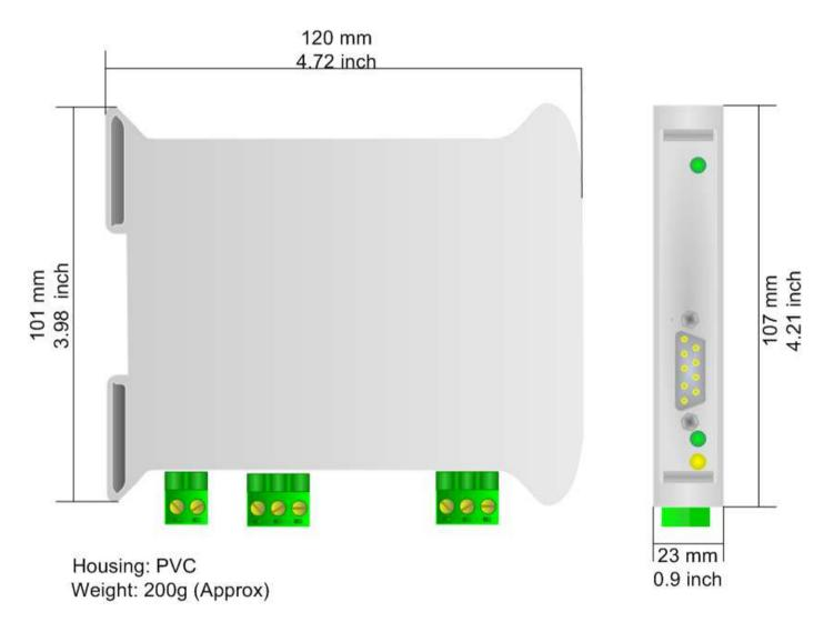
Figure 8: Mechanical dimensions scheme for HD67291-A1
