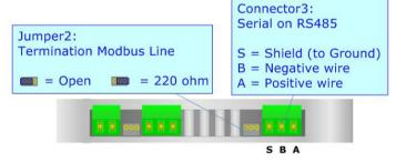
The maximum length of the cable should be 1200m (4000 feet).
