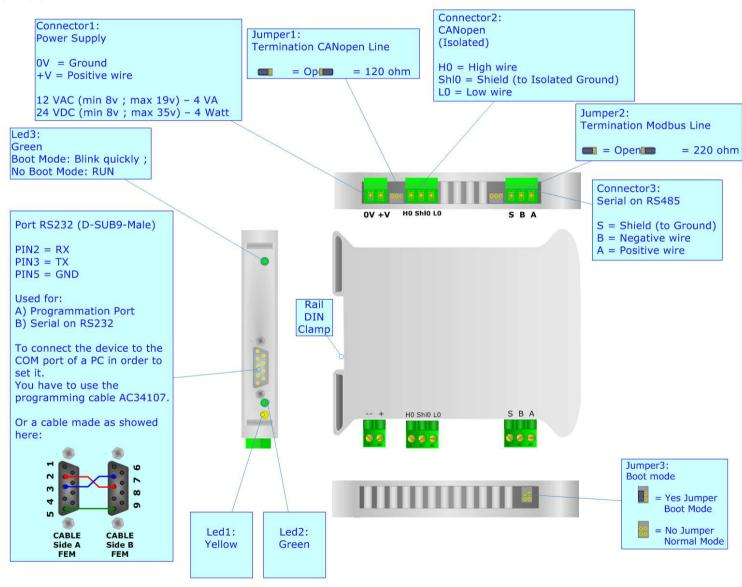
Figure 1: Connection scheme for HD67291-A1
