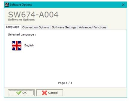
In the section "Connection Options", it is possible to check if there are some updatings of the software compositor in ADFweb.com website. Checking the option "Check Software Update at Start of Program", the SW674-A004 checks automatically if there are updatings when it is launched.
