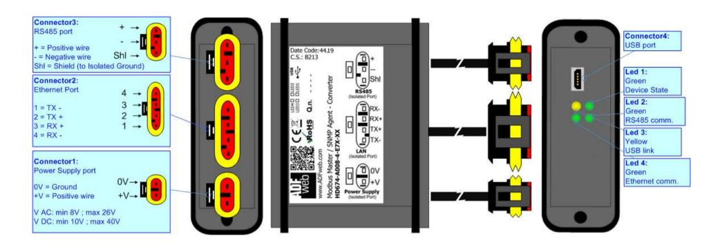
Figure 1d: Connection scheme for HD674-A008-4-E7x-xx
