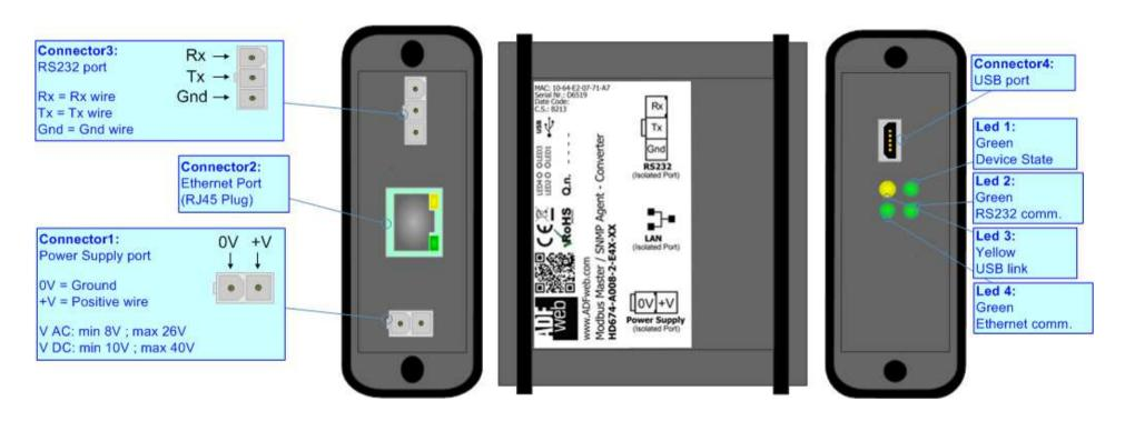
Figure 1a: Connection scheme for HD674-A008-2-E4x-xx
