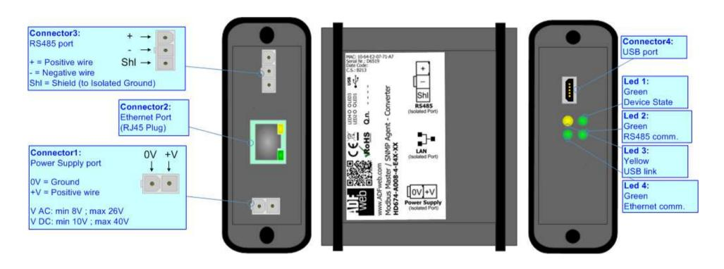
Figure 1c: Connection scheme for HD674-A008-4-E4x-xx
