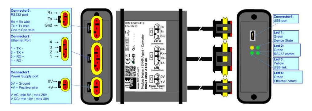
Figure 1b: Connection scheme for HD674-A008-2-E7x-xx
