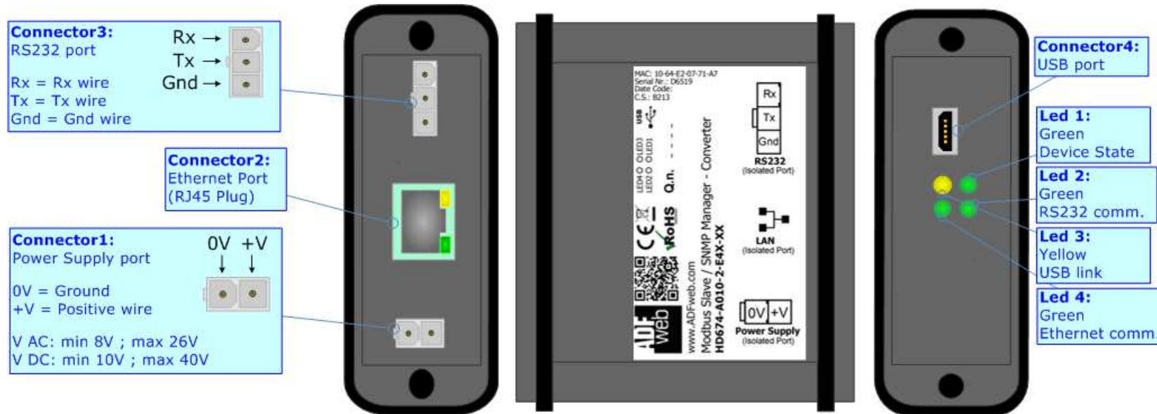
Figure 1a: Connection scheme for HD674-A010-2-E4x-xx
