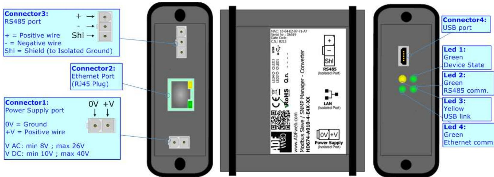
Figure 1c: Connection scheme for HD674-A010-4-E4x-xx
