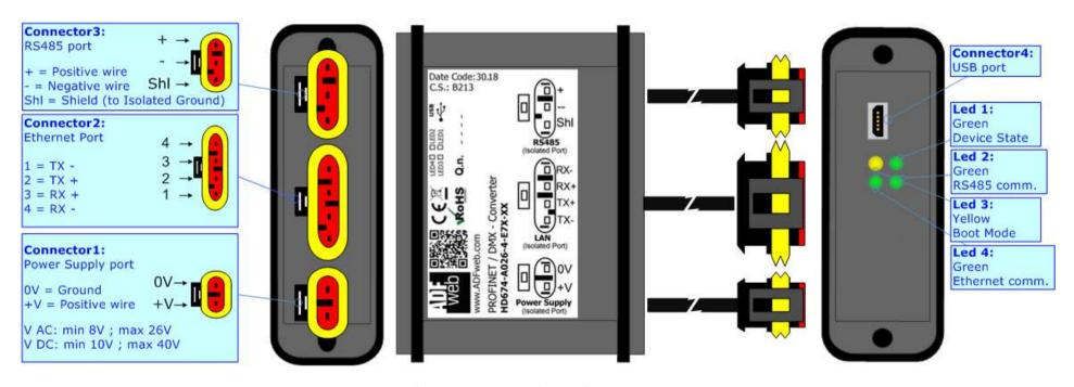
Figure 1b: Connection scheme for HD674-A026-E7x-xx
