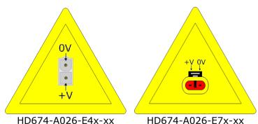
Note: It is possible to use also negative tensions. In this case the polarity must be inverted.
