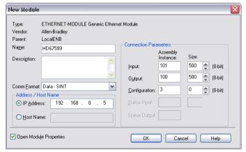
2) Edit the settings of the new Generic Ethernet Module. As shown in the screen shot below, the module was named "HD674-A026" and the IP-address assigned is 192.168.0.5.
