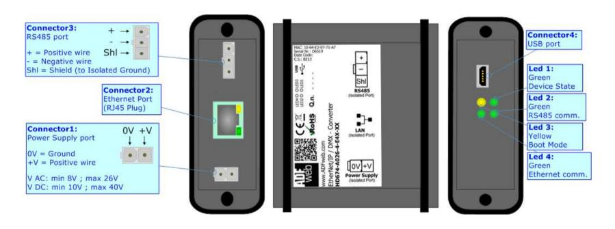
Figure 1a: Connection scheme for HD674-A026-E4x-xx
