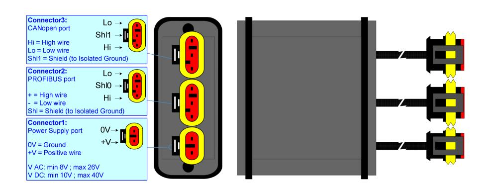
Figure 1-2: Connection scheme for HD67426-E7x-xxx
