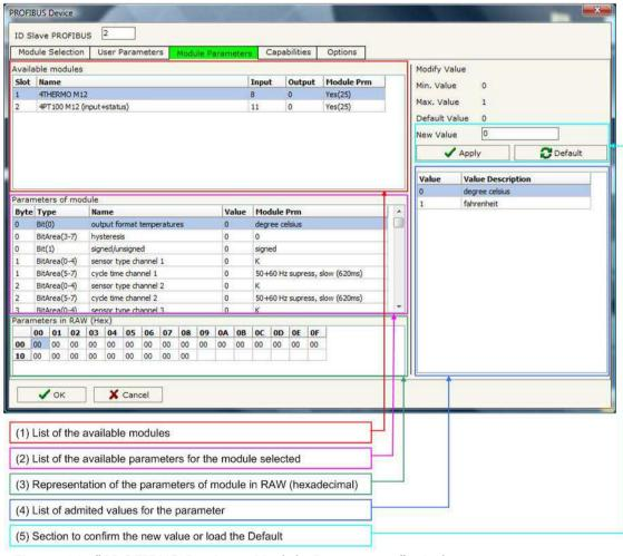
Figure 11: "PROFIBUS Device - Module Parameters" window
