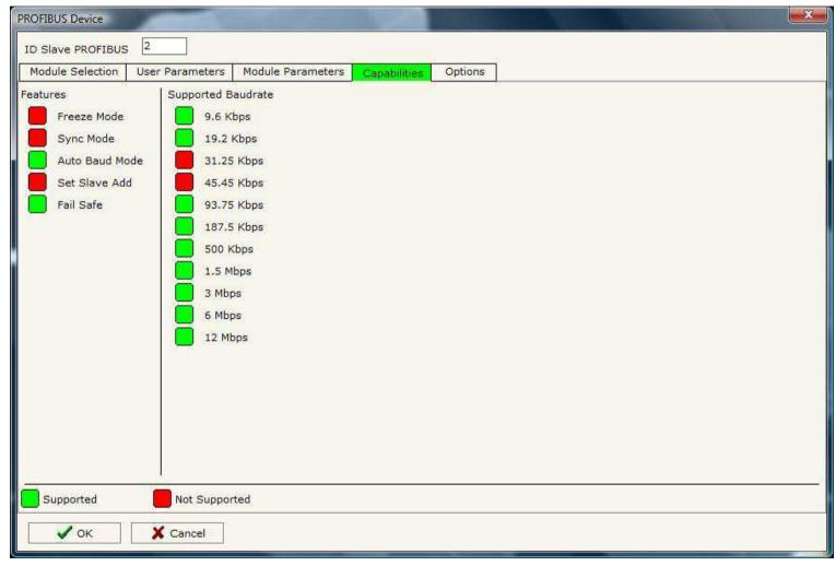
Figure 12: "PROFIBUS Device - Capabilities" window
