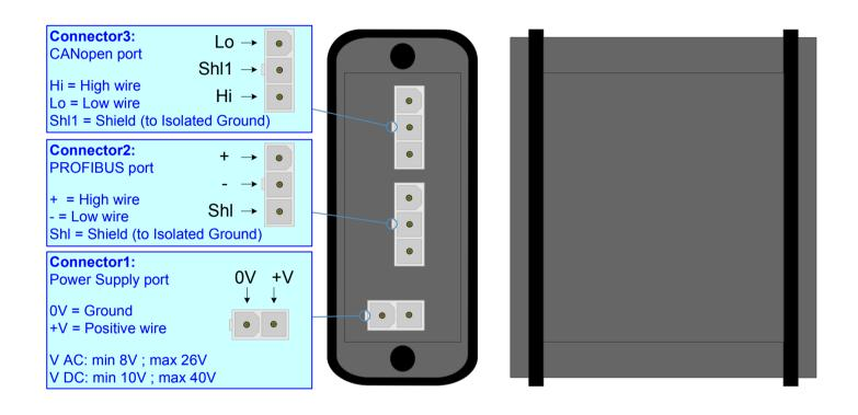
Figure 1-1: Connection scheme for HD67426-E4x-xxx
