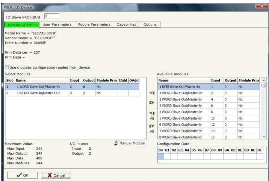
Figure 6: "PROFIBUS Device" window
