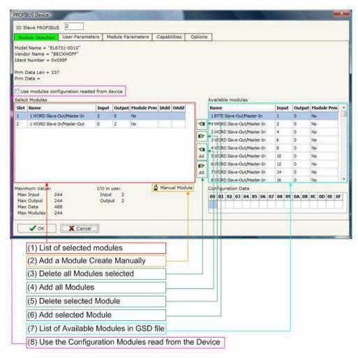
Figure 7: "PROFIBUS Device - Module Selection" window
