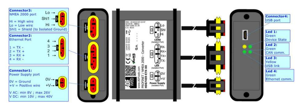
Figure 1b: Connection scheme for HD67459-E7x-xx
