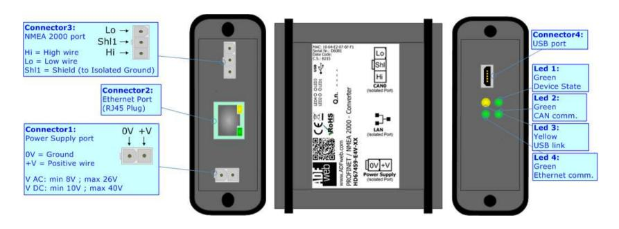
Figure 1a: Connection scheme for HD67459-E4x-xx
