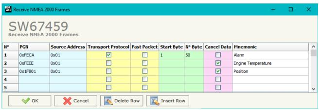
Figure 4: "Receive NMEA 2000 Frames" window
