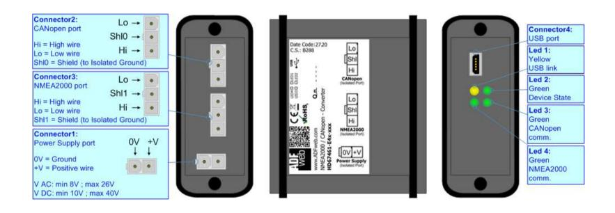
Figure 1a: Connection scheme for HD67461-E4x-xxx
