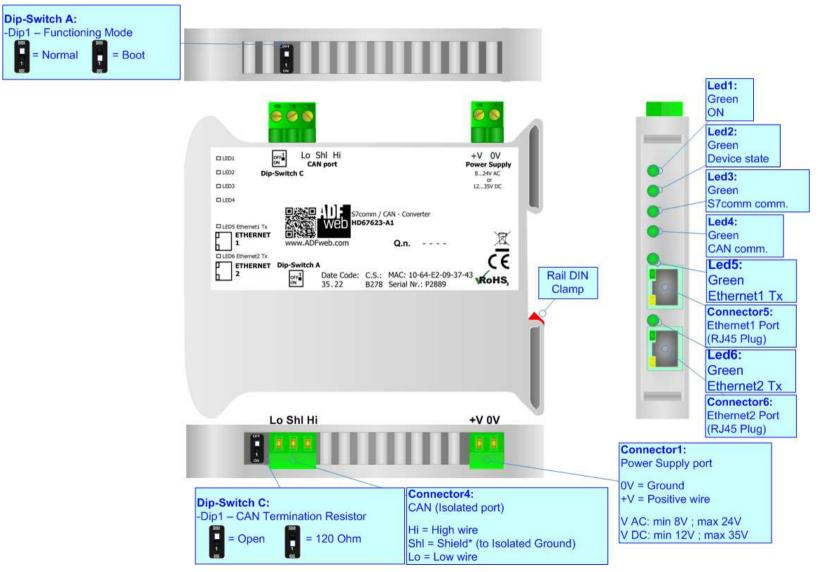
Figure 1: Connection scheme for HD67623-A1
