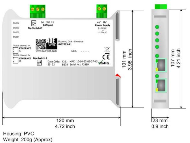
*Figure 9: Mechanical dimensions scheme for HD67623-A1*
