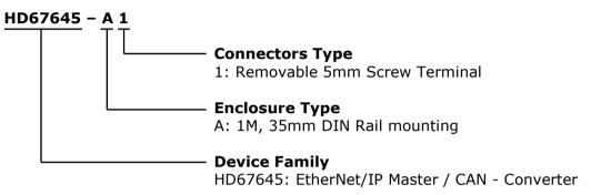
Order Code: **HD67645-A1** - EtherNet/IP Master / CAN – Converter
