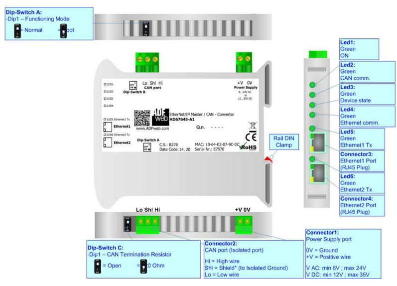
Figure 1: Connection scheme for HD67645-A1
