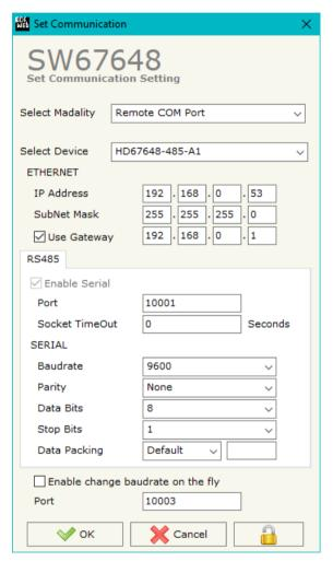
Figure 3: "Devices Setting" window (Remote COM Port)
