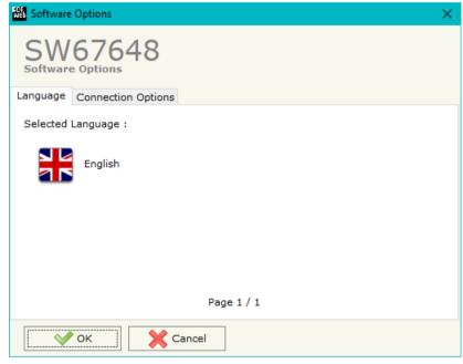
In the section "Connection Options", it is possible to check if there are some updatings of the software compositor in ADFweb.com website. Checking the option "Check Software Update at Start of Program", the SW67648 check automatically if there are updatings when it is launched.
