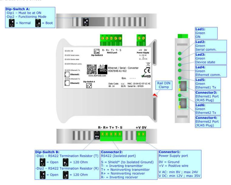
Figure 1c: Connection scheme for HD67648-A1-422
