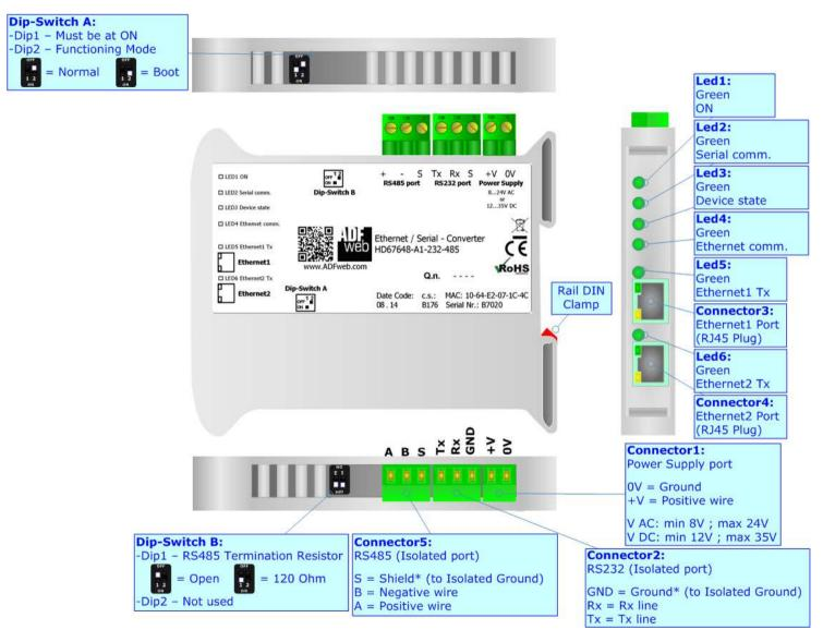
Figure 1d: Connection scheme for HD67648-A1-232-485
