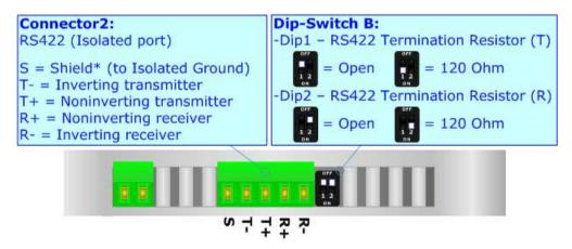
The maximum length of the cable should be 1200m (4000 feet).
