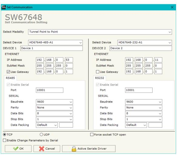
Figure 4: "Devices Setting" window (Tunnel Point to Point)
