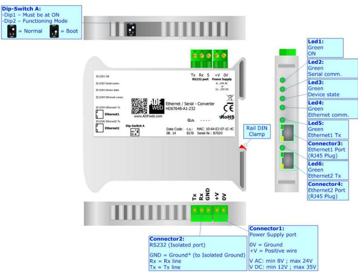
Figure 1a: Connection scheme for HD67648-A1-232
