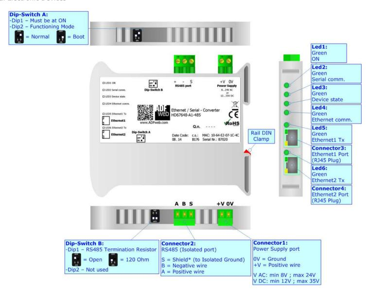
Figure 1b: Connection scheme for HD67648-A1-485
