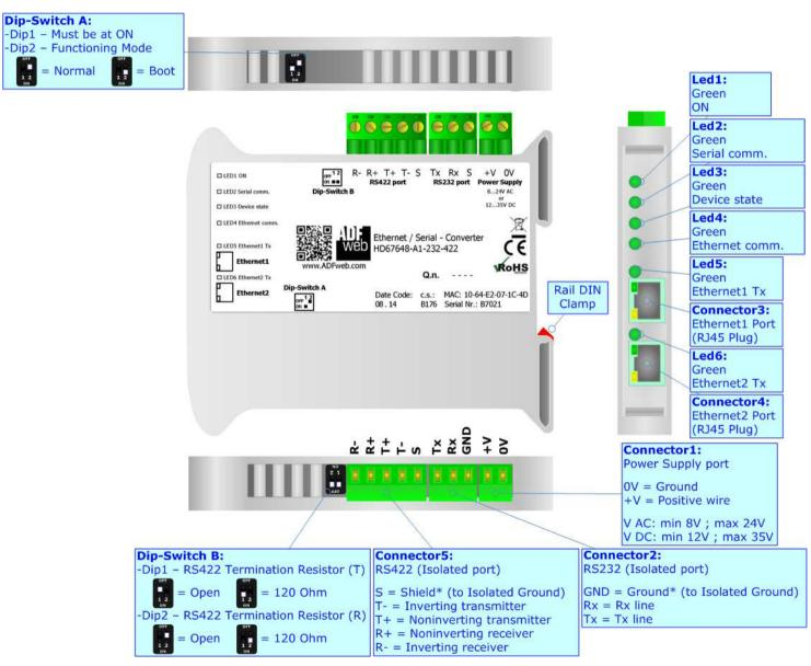
Figure 1e: Connection scheme for HD67648-A1-232-422
