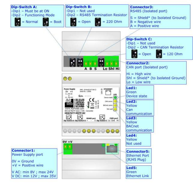
Figure 1c: Connection scheme for HD67677-MSTP-B2
