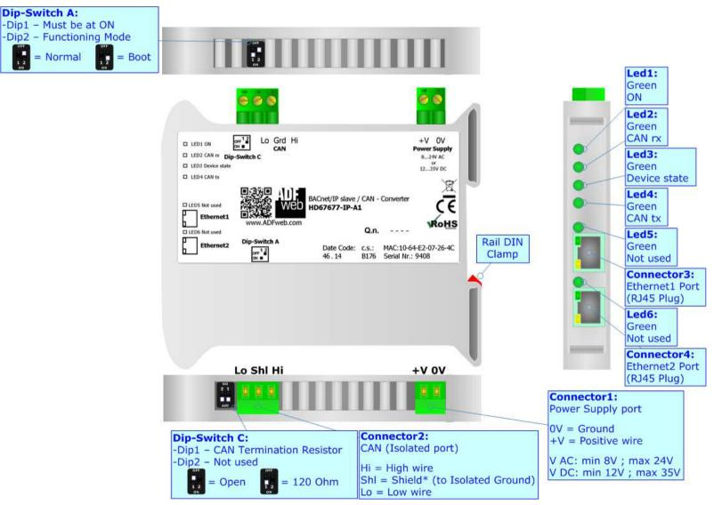
Figure 1a: Connection scheme for HD67677-IP-A1
