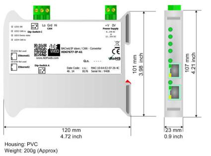
Figure 12a: Mechanical dimensions scheme for HD67677-IP-A1
