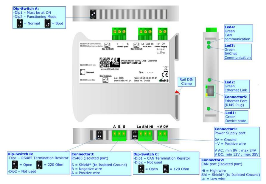
Figure 1b: Connection scheme for HD67677-MSTP-A1
