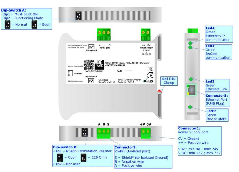
Figure 1b: Connection scheme for HD67722-MSTP-A1
