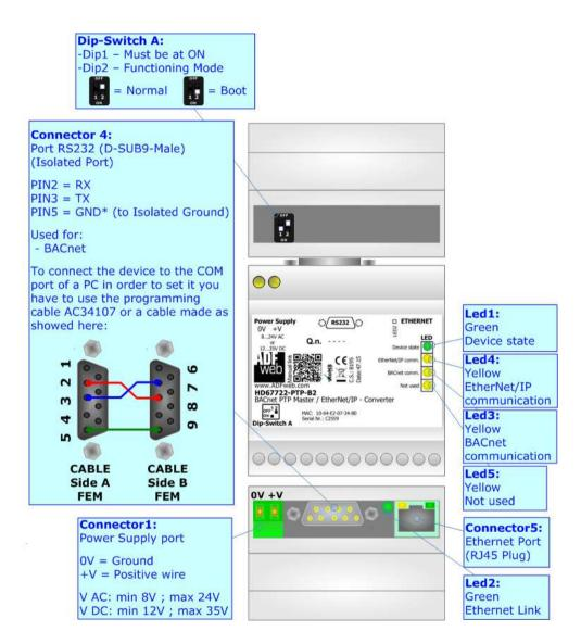
Figure 1e: Connection scheme for HD67722-PTP-B2
