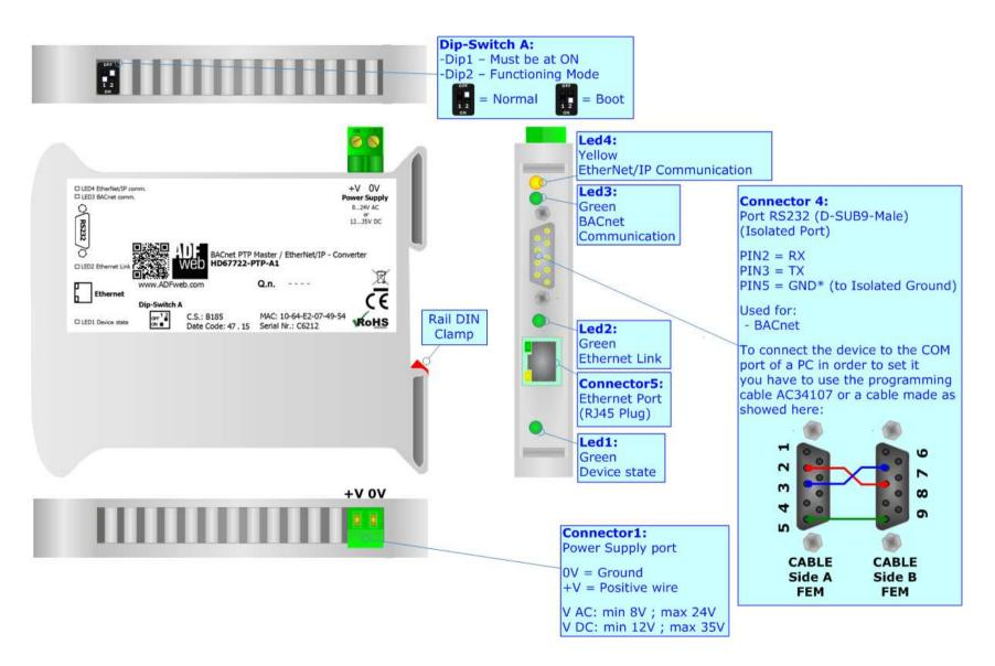
Figure 1d: Connection scheme for HD67722-PTP-A1
