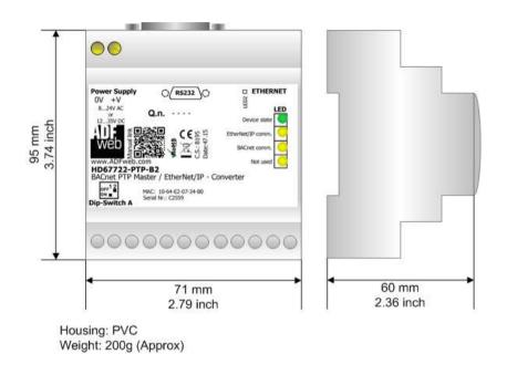
Figure 7e: Mechanical dimensions scheme for HD67722-PTP-B2
