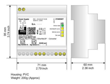
Figure 7d: Mechanical dimensions scheme for HD67722-MSTP-B2
