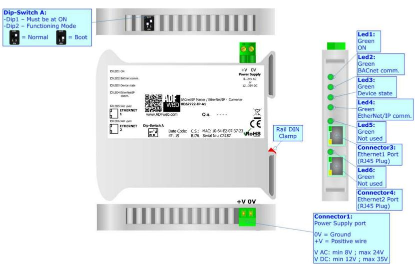
Figure 1a: Connection scheme for HD67722-IP-A1
