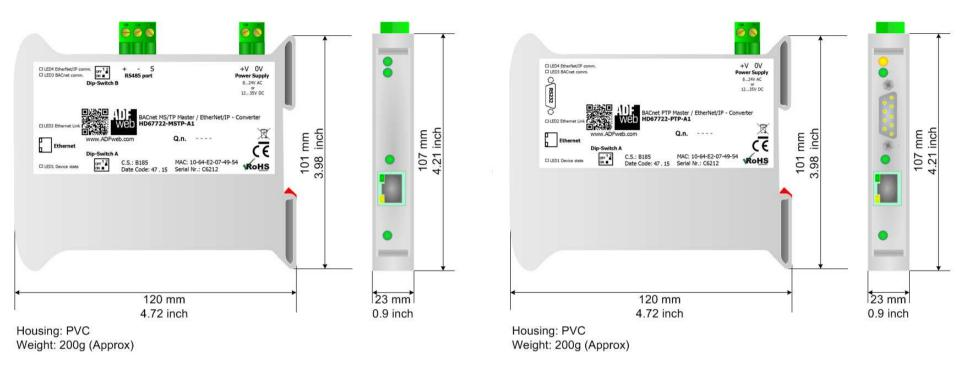
Figure 7b: Mechanical dimensions scheme for HD67722-MSTP-A1
