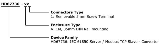
Order Code: **HD67736-A1** - IEC 61850 Server / Modbus TCP Slave - Converter
