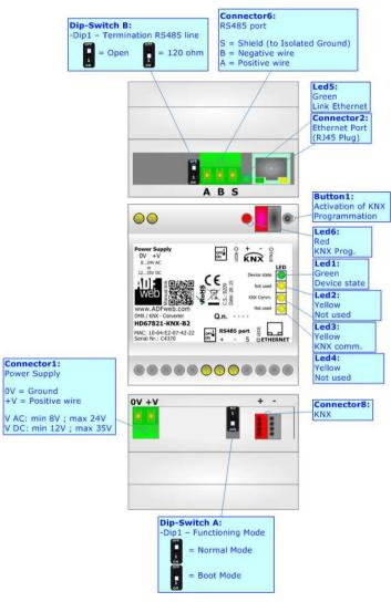
Figure 1: Connection scheme for HD67821-KNX-B2
