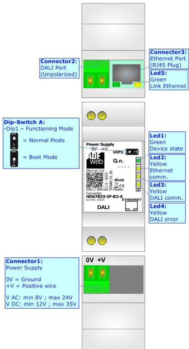
Figure 1a: Connection scheme for HD67833-IP-B2
