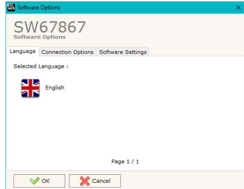
In the section “Connection Options”, it is possible to check if there are some updates of the software compositor in ADFweb.com website. Checking the option “**Check Software Update at Start of Program**”, the SW67867 check automatically if there are updates when it is launched.
