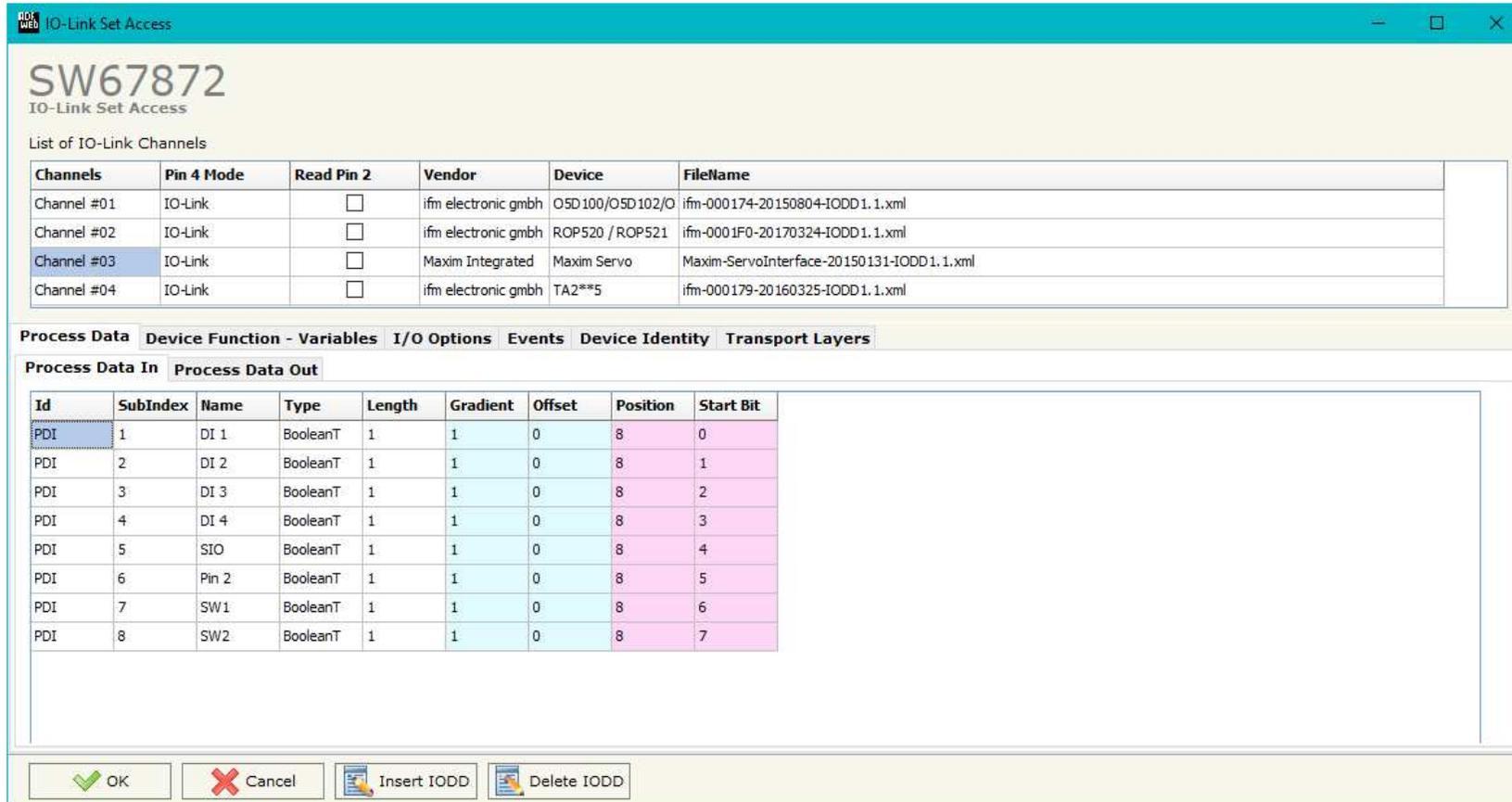
Figure 4: “IO-Link Set Access” window
