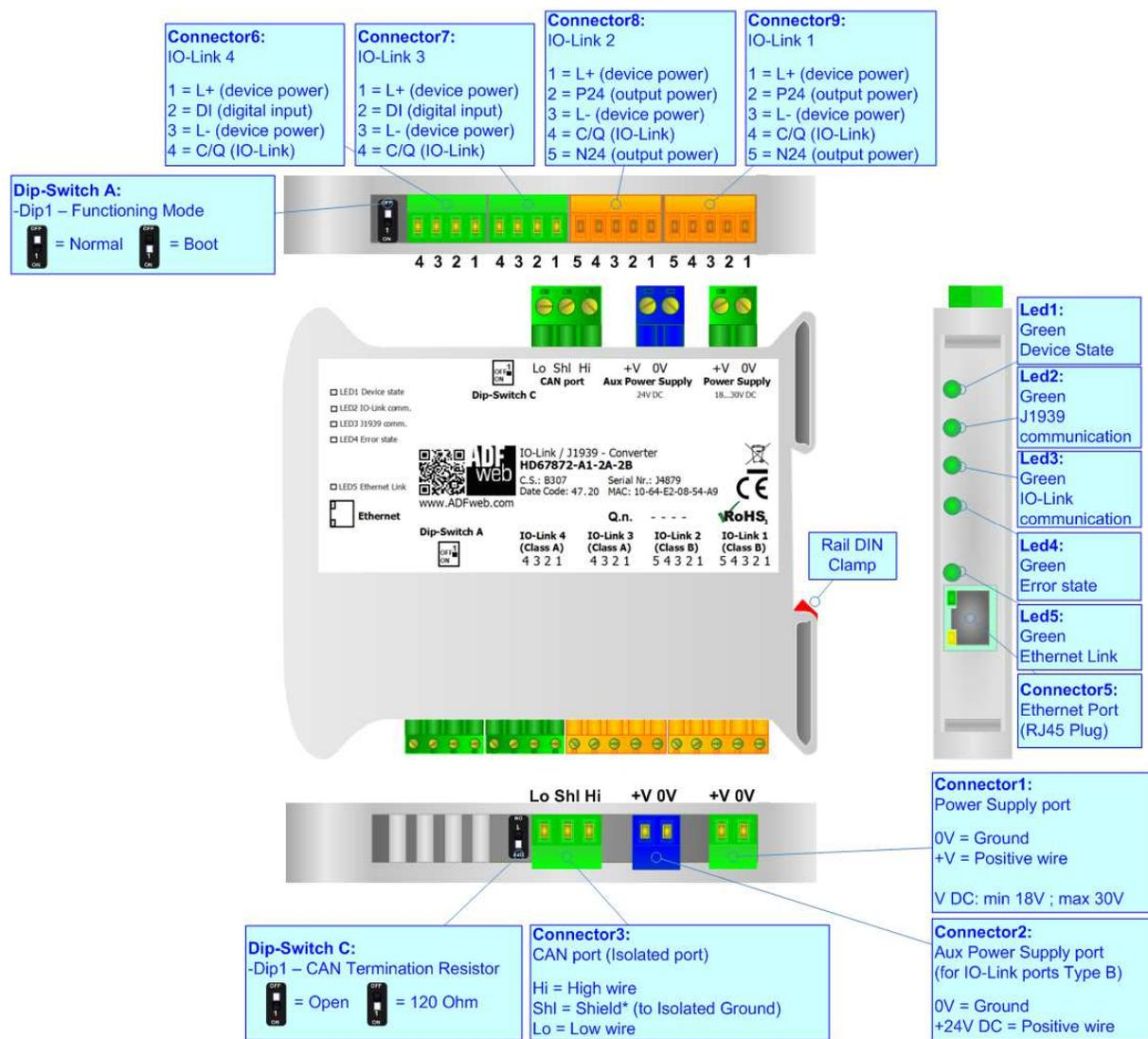
Figure 1d: Connection scheme for HD67872-A1-2A-2B
