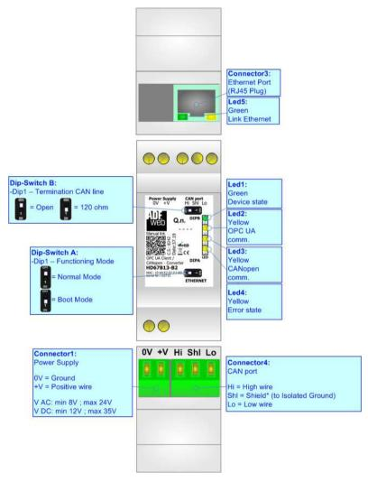
Figure 1: Connection scheme for HD67B13-B2
