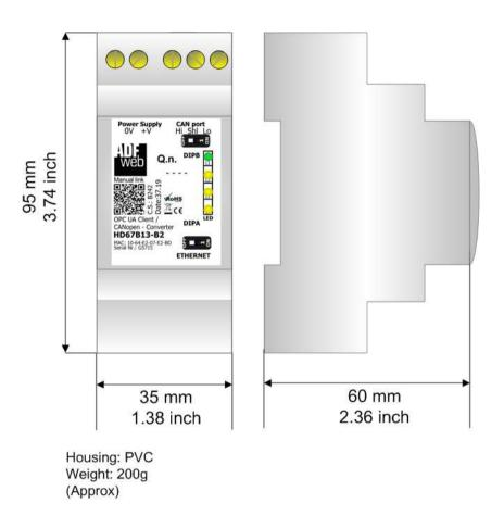
Figure 15: Mechanical dimensions scheme for HD67B13-B2
