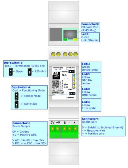
Figure 1: Connection scheme for HD67B37-B2
