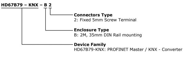
Order Code: HD67B79-KNX-B2 - PROFINET Master / KNX - Converter
