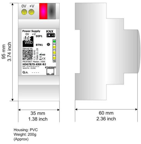
Figure 9: Mechanical dimensions scheme for HD67B79-KNX-B2
