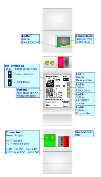
Figure 1: Connection scheme for HD67B79-KNX-B2
