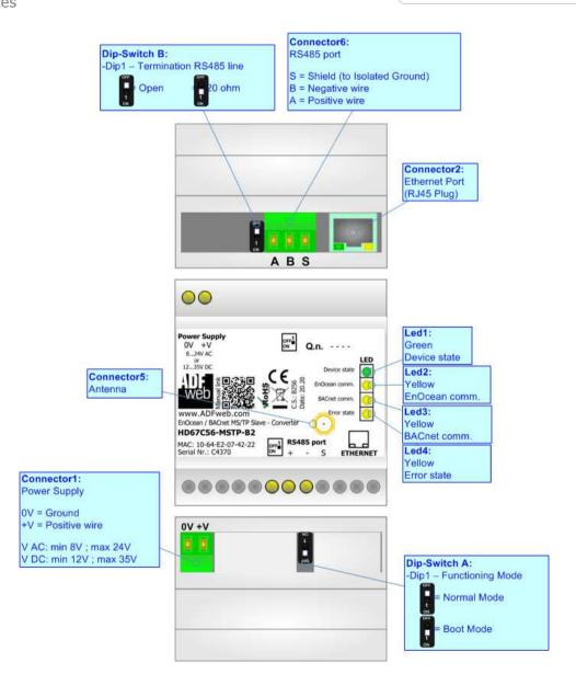
Figure 1b: Connection scheme for HD67C56-MSTP-B2
