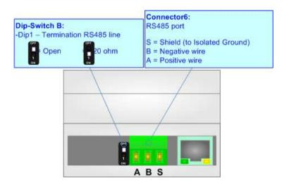
The maximum length of the cable should be 1200m (4000 feet).
