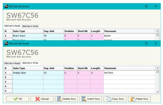
Figure 7: "BACnet Set Access" window
