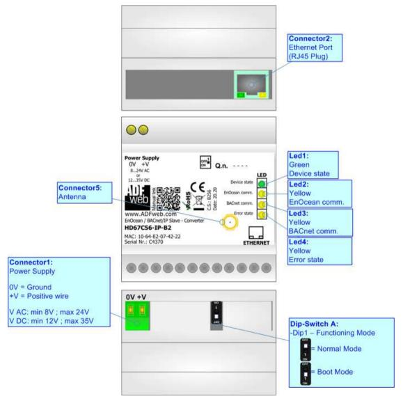
Figure 1a: Connection scheme for HD67C56-IP-B2
