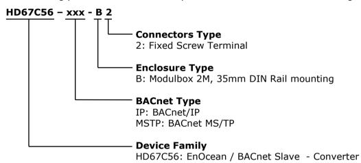
Order Code: **HD67C56-IP-B2** - EnOcean / BACnet/IP Slave - Converter
