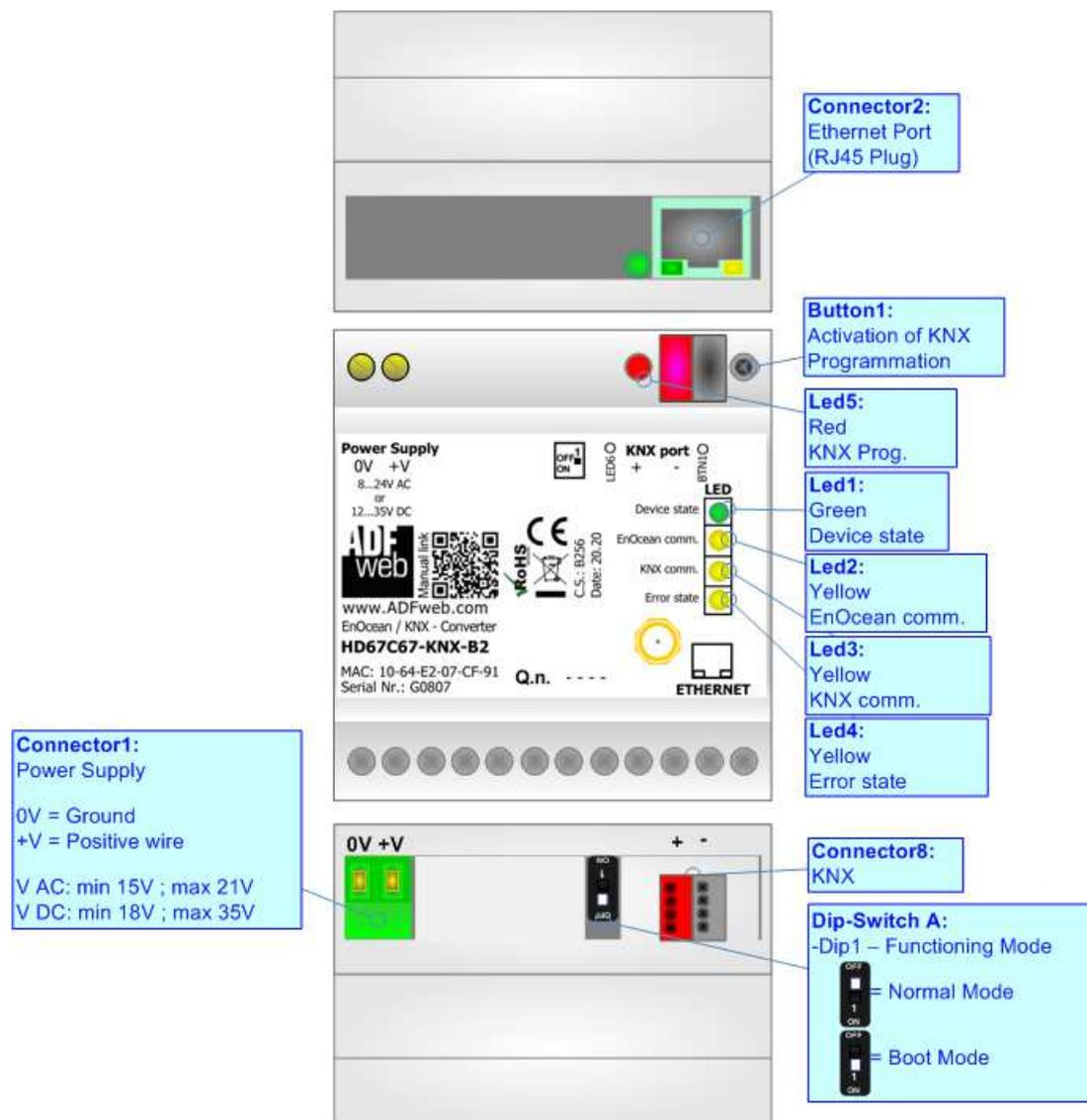
Figure 1: Connection scheme for HD67C67-B2
