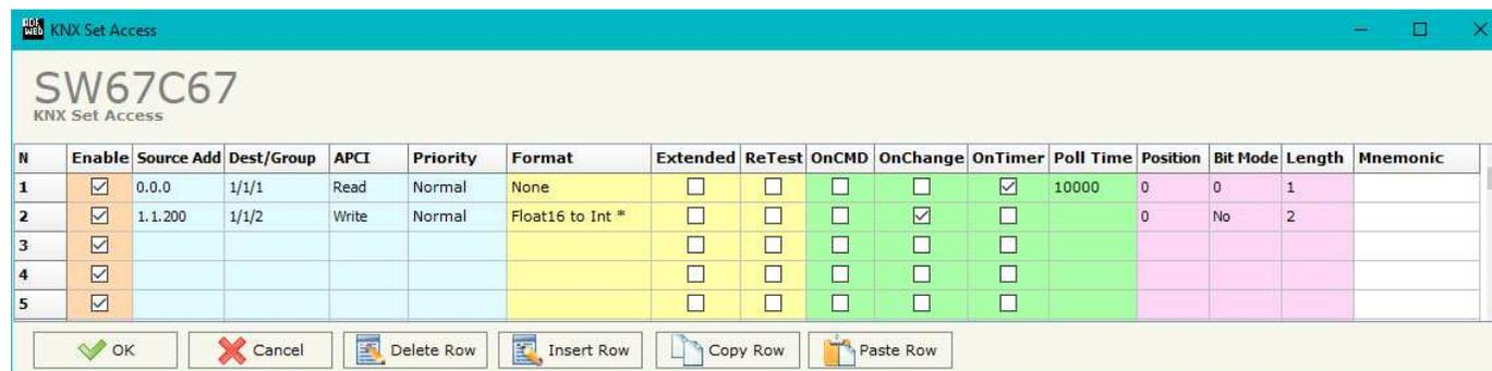
Figure 7: **“KNX Set Access”** window
