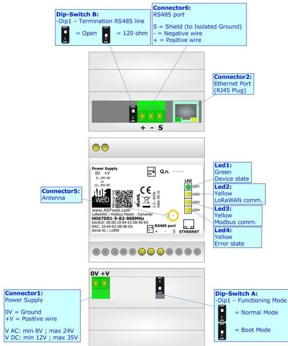
Figure 1b: Connection scheme for HD67D01-5-B2-xxxMHz
