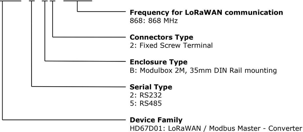
Order Code: **HD67D01-2-B2-868MHz** - LoRaWAN / Modbus Master – Converter (RS232)
