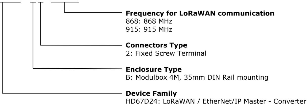
Order Code: **HD67D24-B2-868MHz** - LoRaWAN / EtherNet/IP Master – Converter
