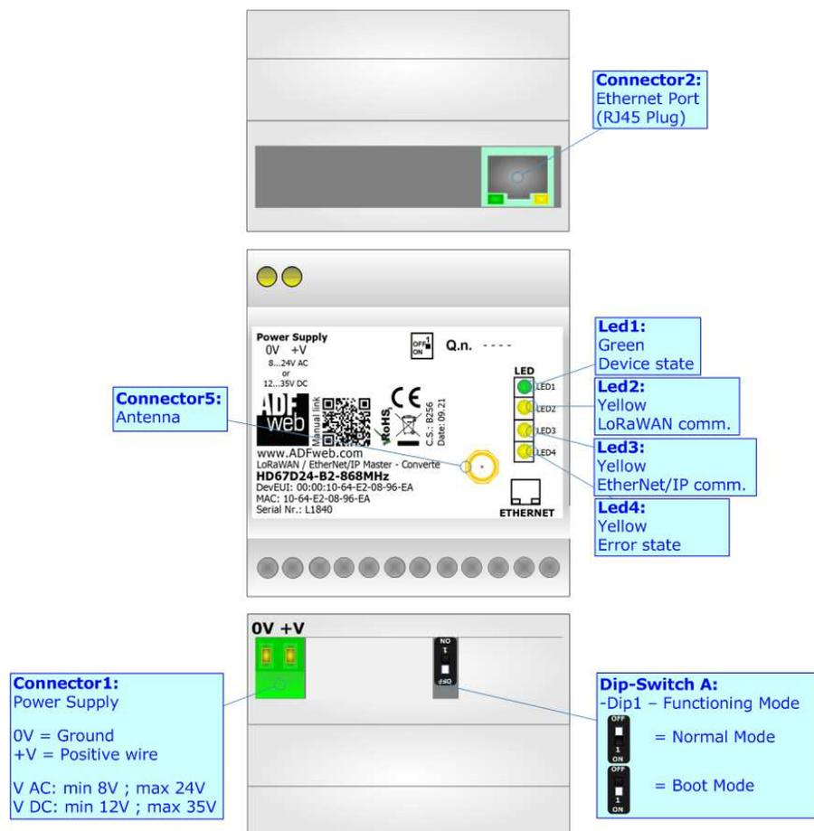
Figure 1: Connection scheme for HD67D24-B2-xxxMHz
