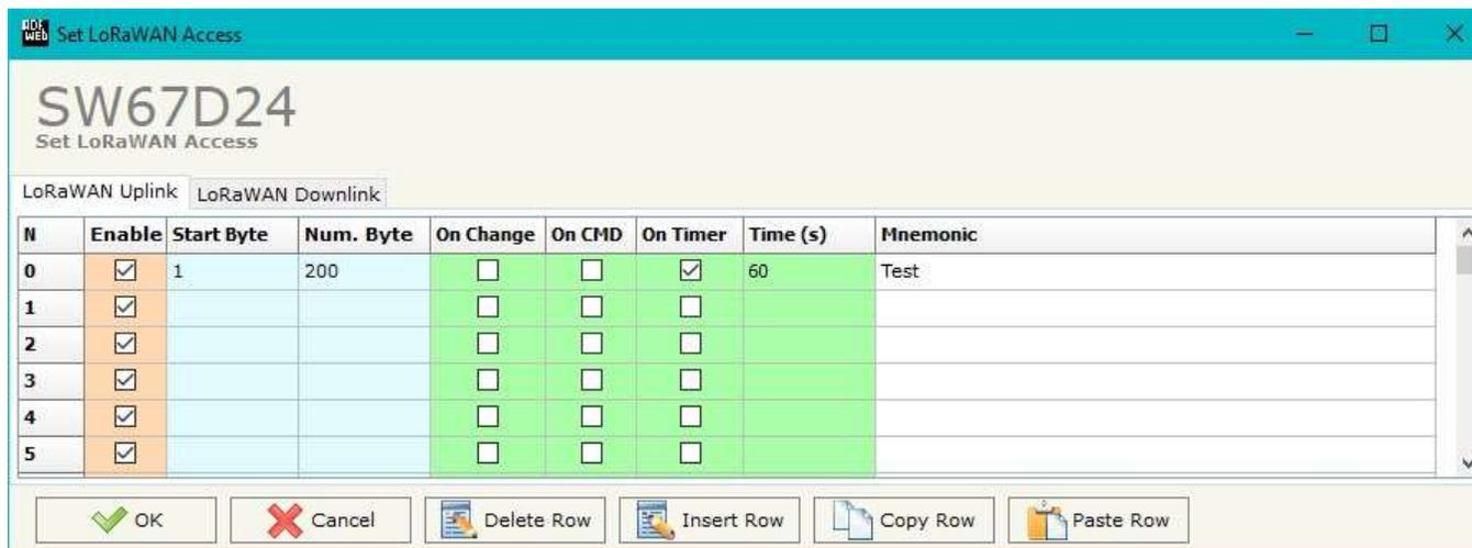
Figure 4a: “LoRaWAN Access → LoRaWAN Uplink” window
