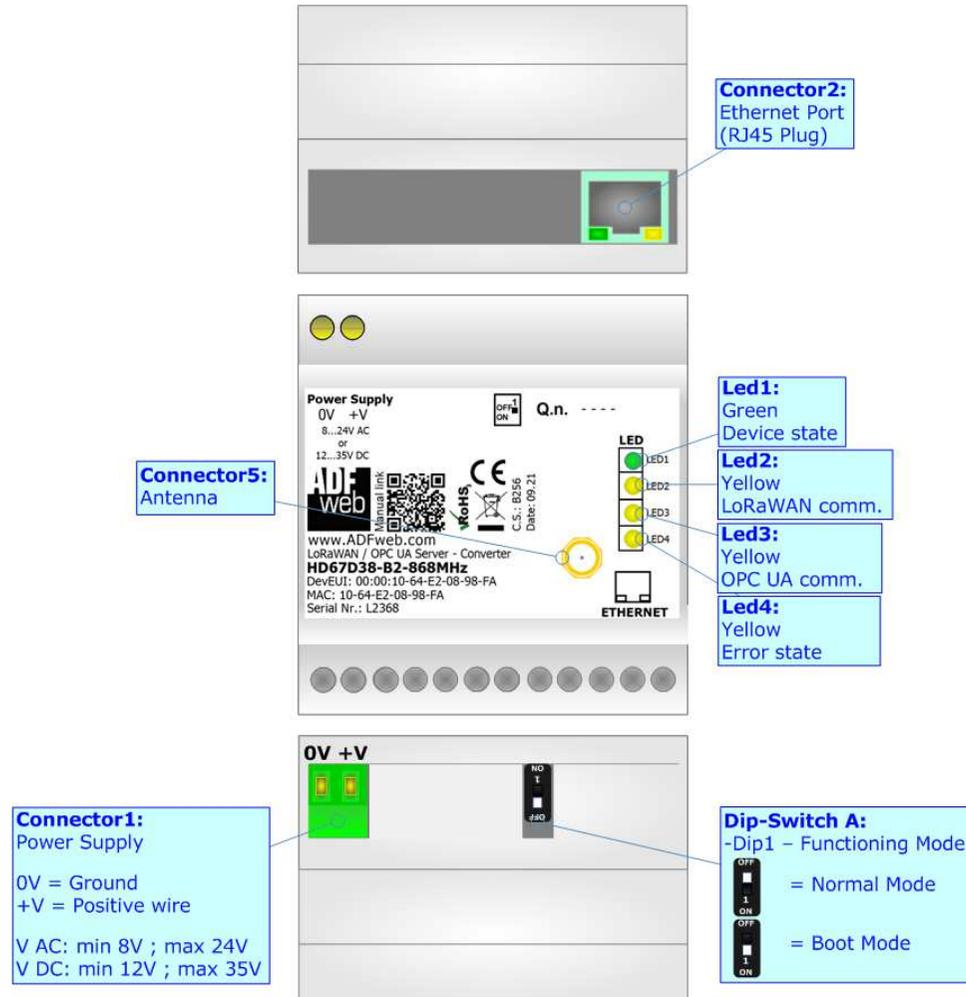
Figure 1: Connection scheme for HD67D38-B2-xxxMHz
