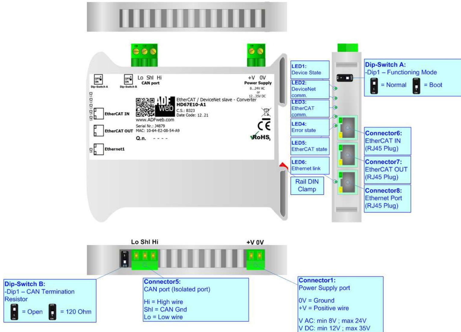
Figure 1: Connection scheme for HD67E10-A1
