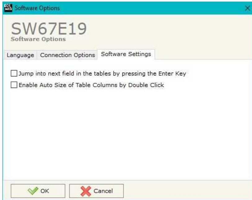
In the section "Software Settings", it is possible to enable/disable some keyboard's commands for an easier navigation inside the tables contained in the different sections of the software.
