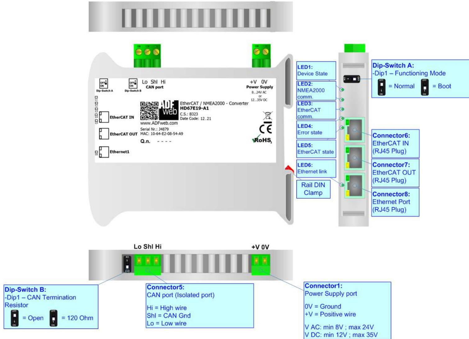
Figure 1: Connection scheme for HD67E19-A1
