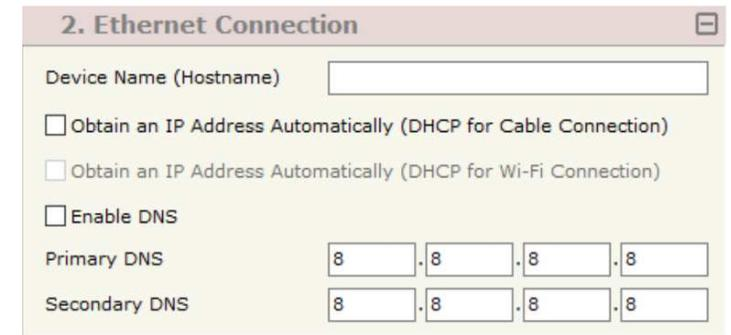
Figure 3c: "Set Communication → Ethernet connection" window
