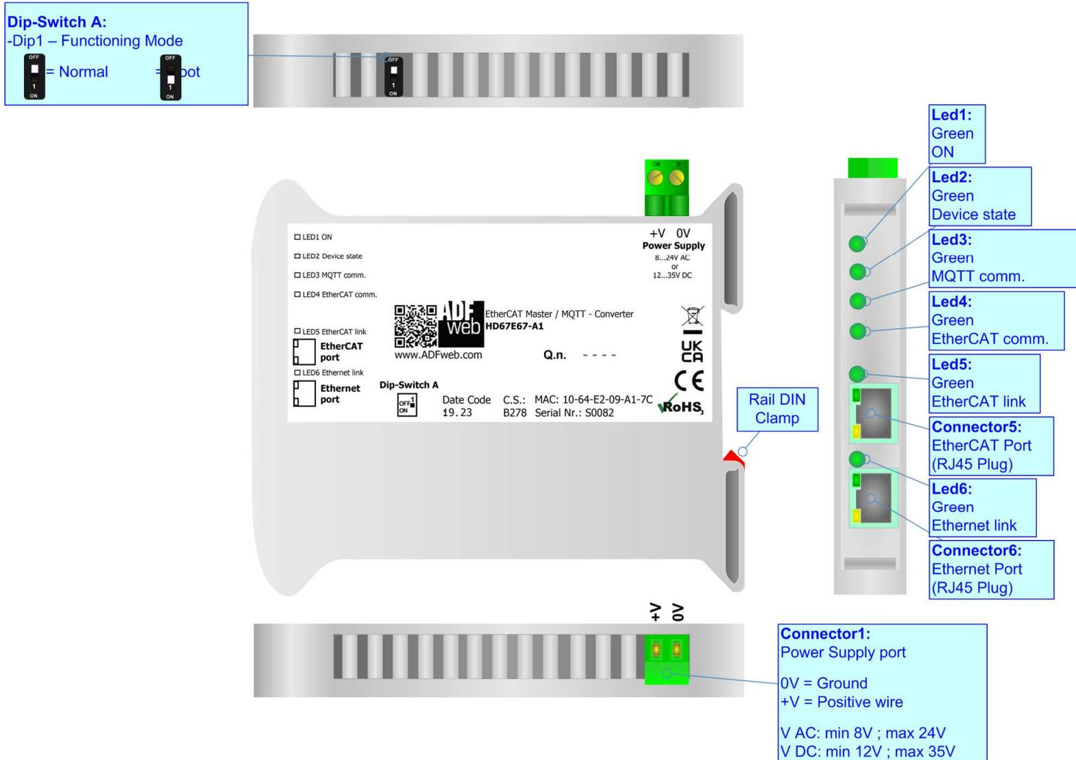
Figure 1: Connection scheme for HD67E67-A1
