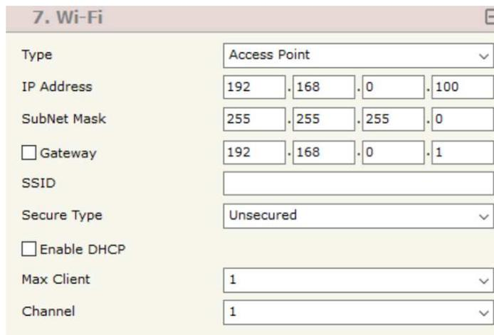
Figure 3h: "Set Communication → Wi-Fi (Access Point)" window
