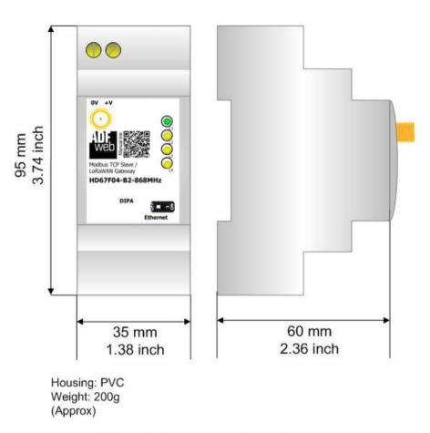
Figure 7: Mechanical dimensions scheme for HD67F04-B2-xxxMHz
