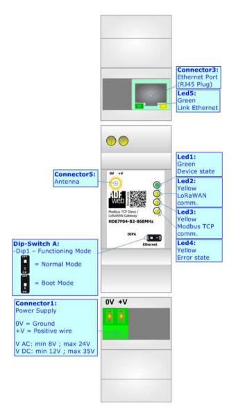
Figure 1: Connection scheme for HD67F04-B2-xxxMHz
