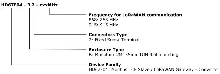
Order Code: **HD67F04-B2-868MHz** - Modbus TCP Slave / LoRaWAN Gateway - Converter (868MHz)
