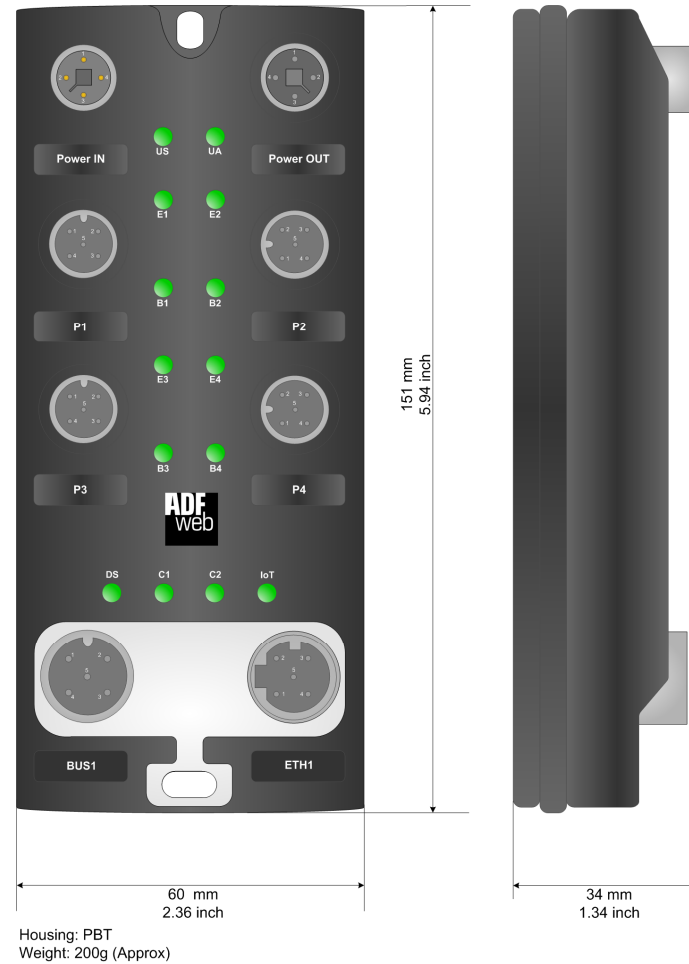
Figure 10a: Mechanical dimensions scheme for HD67X4Px
