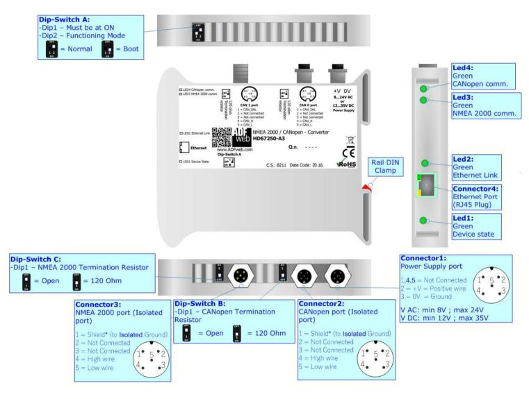
Figure 1b: Connection scheme for HD67250-A3
