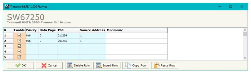
Figure 7a: "Transmit NMEA 2000 Frames Set Access" window
