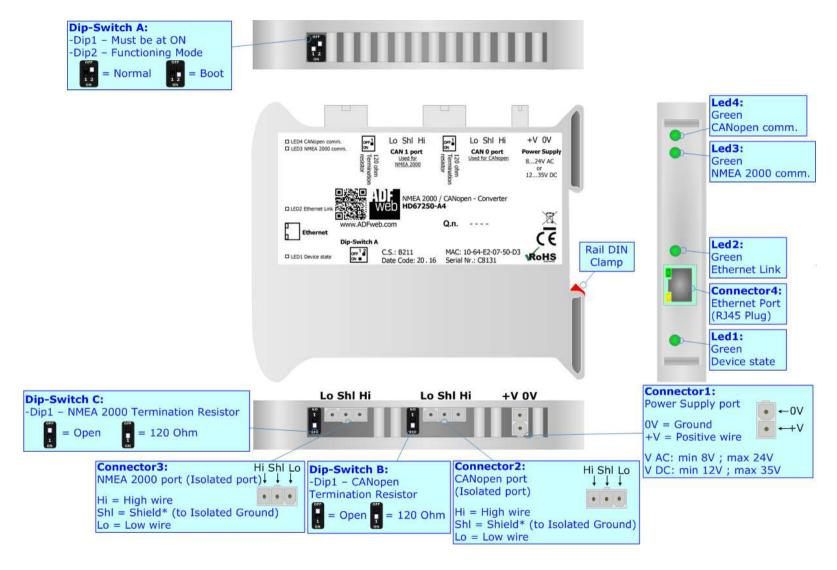
Figure 1c: Connection scheme for HD67250-A4
