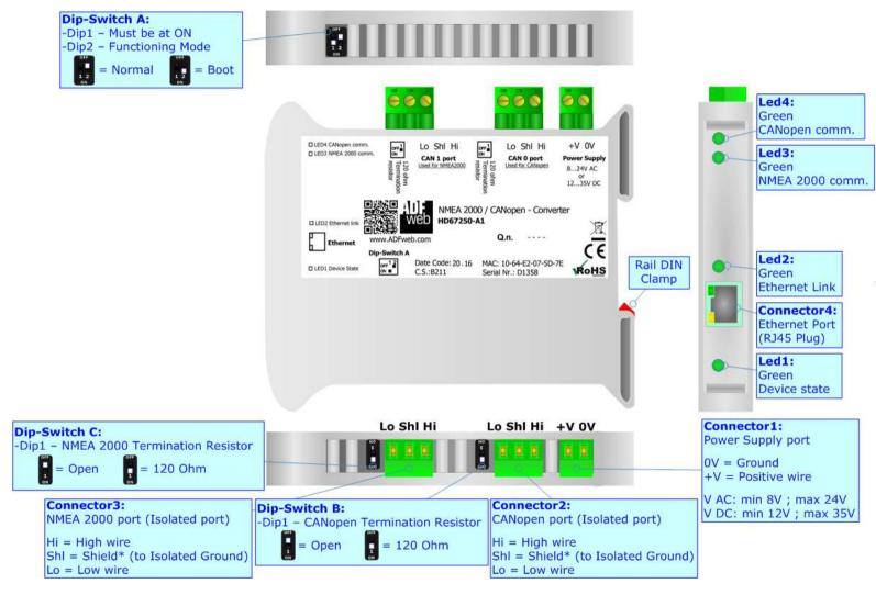
Figure 1a: Connection scheme for HD67250-A1
