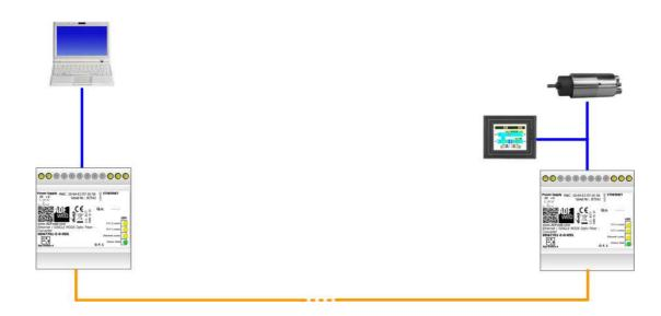
2) <u>Single Loop</u>: more devices will be connected serially using Optical Fiber, closing the network in a Ring.
