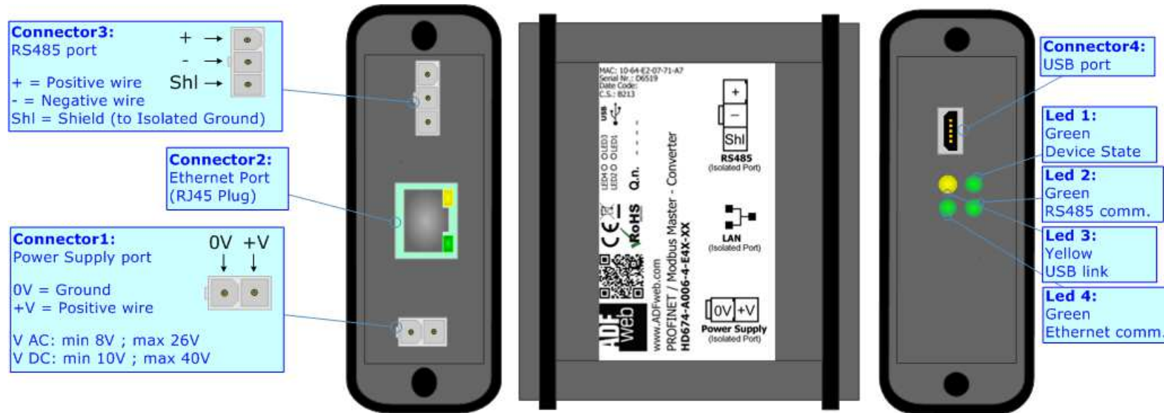
Figure 1c: Connection scheme for HD674-A006-4-E4x-xx
