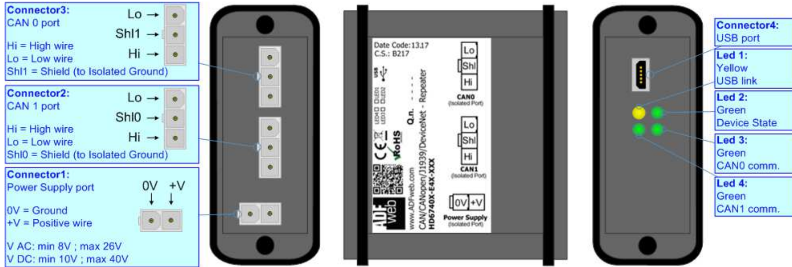
Figure 1a: Connection scheme for HD6740x-E4x-xxx
