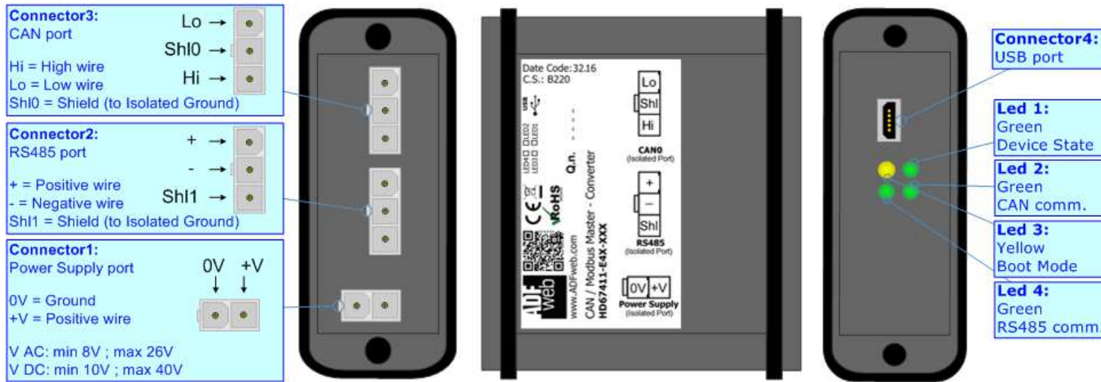
Figure 1a: Connection scheme for HD67411-E4x-xxx
