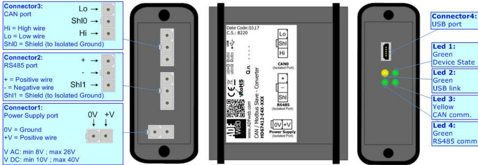
Figure 1a: Connection scheme for HD67412-E4x-xxx
