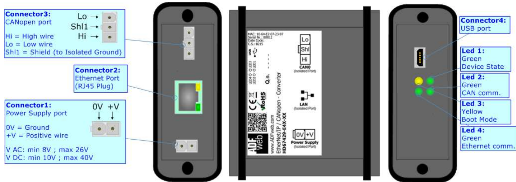
Figure 1a: Connection scheme for HD67429-E4x-xx
