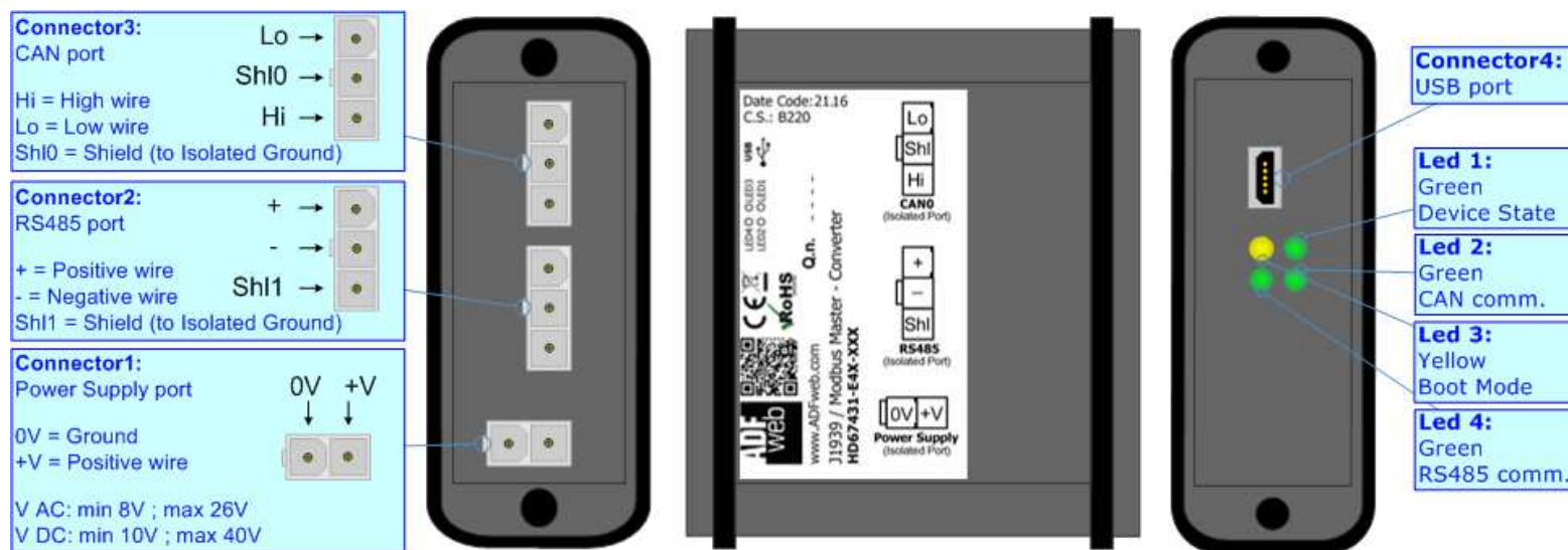
Figure 1a: Connection scheme for HD67431-E4x-xxx
