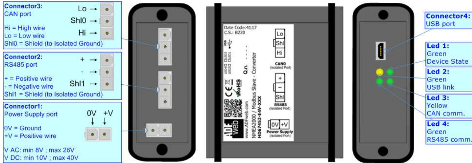
Figure 1a: Connection scheme for HD67452-E4x-xxx
