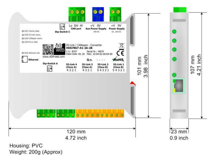
Figure 18: Mechanical dimensions scheme for HD67867-A1-xx
