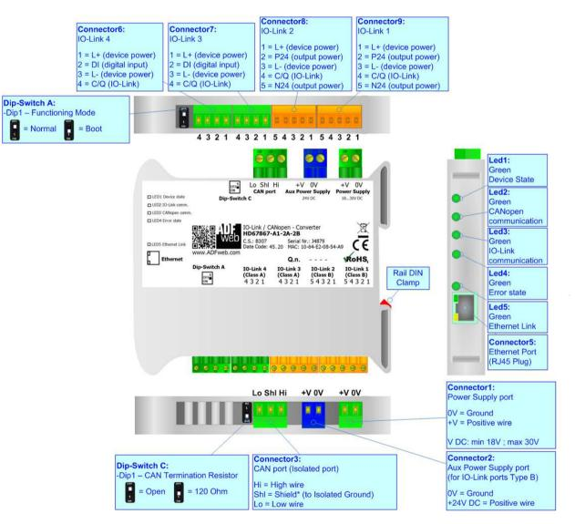
Figure 1d: Connection scheme for HD67867-A1-2A-2B
