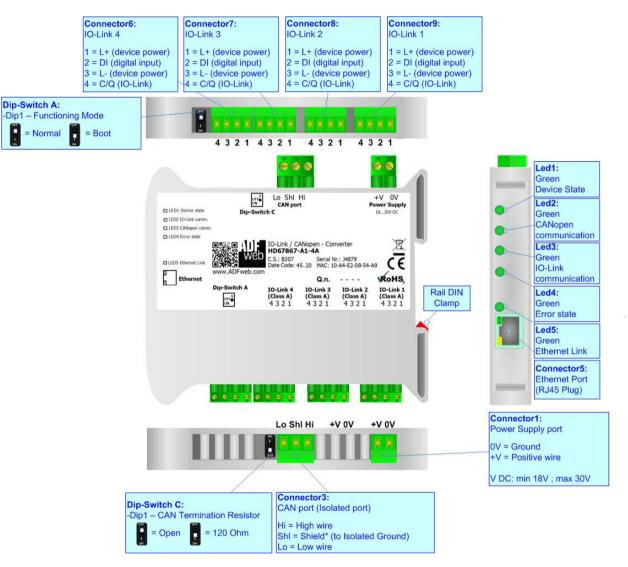
Figure 1b: Connection scheme for HD67867-A1-4A
