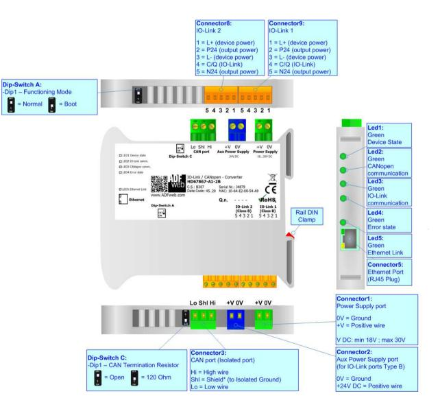
Figure 1c: Connection scheme for HD67867-A1-2B
