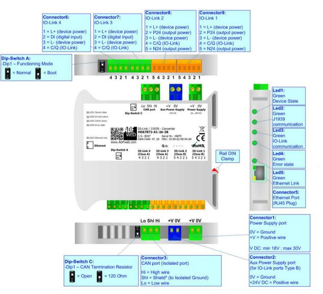
Figure 1d: Connection scheme for HD67872-A1-2A-2B
