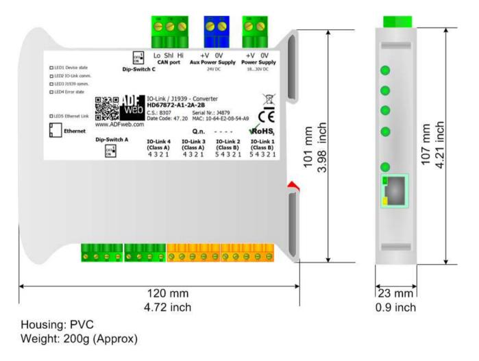
Figure 17: Mechanical dimensions scheme for HD67872-A1-xx
