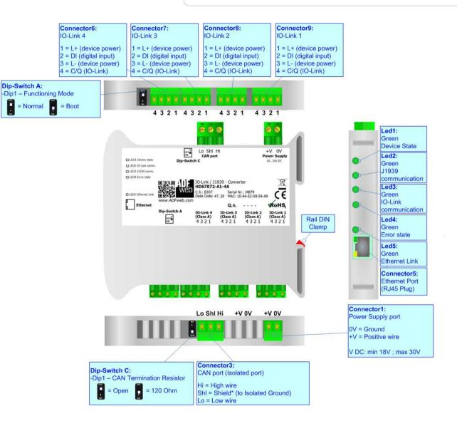
Figure 1b: Connection scheme for HD67872-A1-4A
