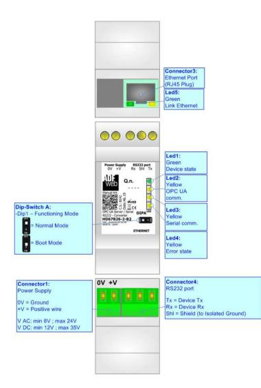
Figure 1a: Connection scheme for HD67B26-2-B2
