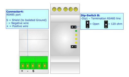
The maximum length of the cable should be 1200m (4000 feet).
