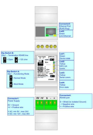
Figure 1b: Connection scheme for HD67B26-5-B2
